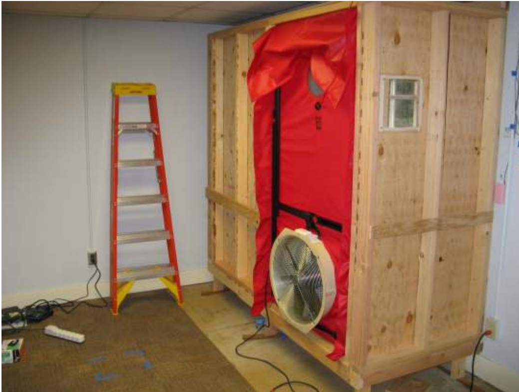
Figure 4, Blower Door Testing in Meter Chamber
